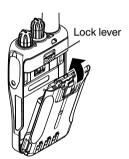
2 To remove the battery pack, push the lock lever up, then pull the battery pack away from the transceiver.
